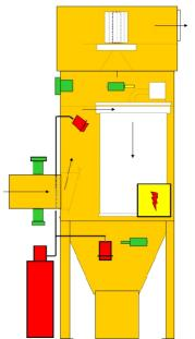
Detection with spark detector, integrated in pipe work, heat detector in hopper plus heat and spark detectors in clean gas section
